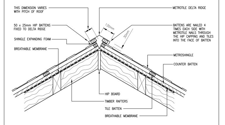
NOTE:- SECTION THROUGH HIP DRAWN FOR A RAFTER PITCH OF 30°
