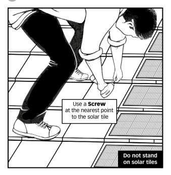
Stand on the nose of the Qube tile (where the batten goes) and nail each Qube tile in the front edge at its highest point (treading on the tiles keeps them nice and tight on the laps!). On the Qube tiles adjacent to eQube solar tiles, use a screw at the nearest point to the eQube solar tile. This allows the solar tile to be removed easilly for maintenance purposes.
