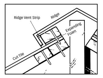
You are now ready to attach the Ridge Vent Strip and the Ridge. Place the Ridge Vent Strip between the batten and the Ridge and nail through the Ridge into the top batten as shown.
