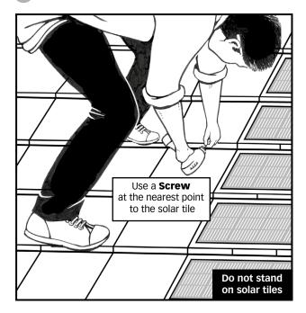
Stand on the nose of the Qube tile (where the batten goes) and nail each Qube tile in the front edge at its highest point (treading on the tiles keeps them nice and tight on the laps!). On the Qube tiles adjacent to eQube solar tiles, use a screw at the nearest point to the eQube solar tile. This allows the solar tile to be removed easilly for maintenance purposes.
